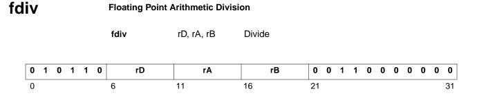
The floating point value in rB is divided by the floating point value in rA and the result is placed into register rD.
